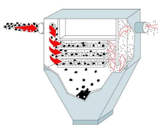
Settling trays can be used to improve removal efficiency.
