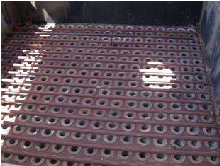
Photo of snap ring and a diagram of a snap ring and tube sheet
