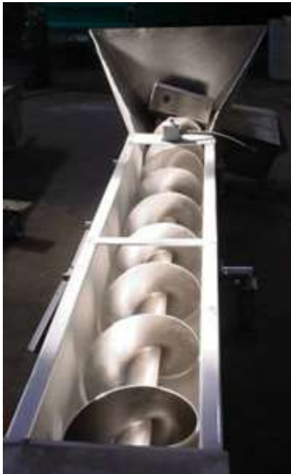
Screw conveyor hopper discharge
