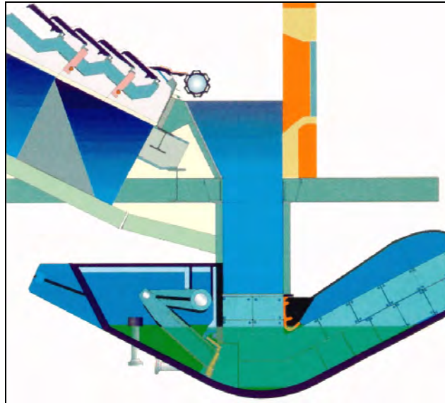
Figure 2.5: Example of a type of ash remover used at a grate incinerator Source [1, UBA, 2001]
