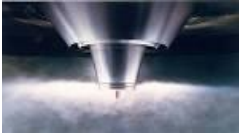
Atomization of lime slurry
