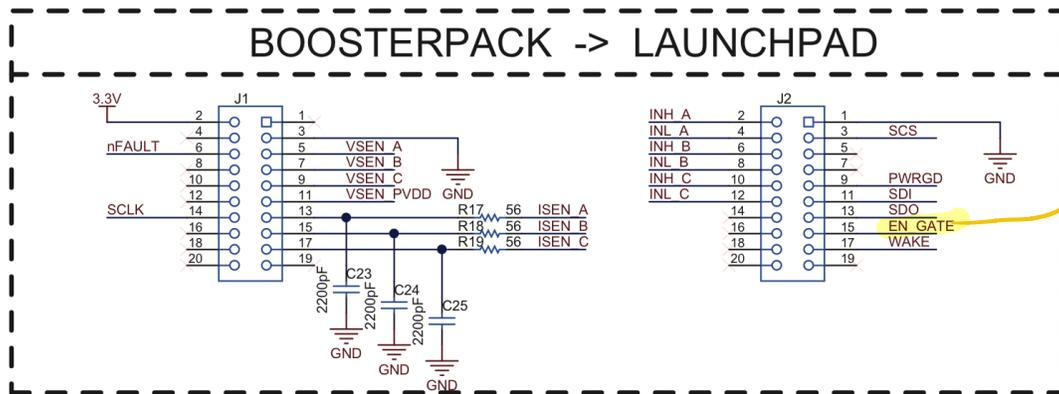
Figure 2. BoosterPack Header Signals
