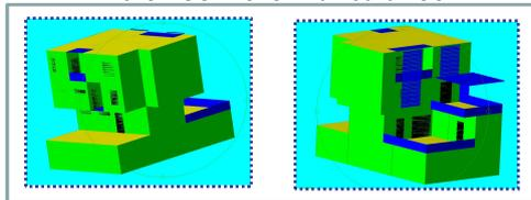
*Lumped resistance-capacity model*
