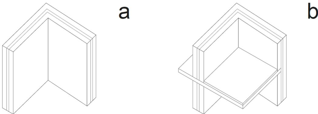
**Figure 2.** (a) Linear and (b) point thermal bridge.
