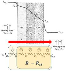
Temperature factor at the internal surface for plane building elements
