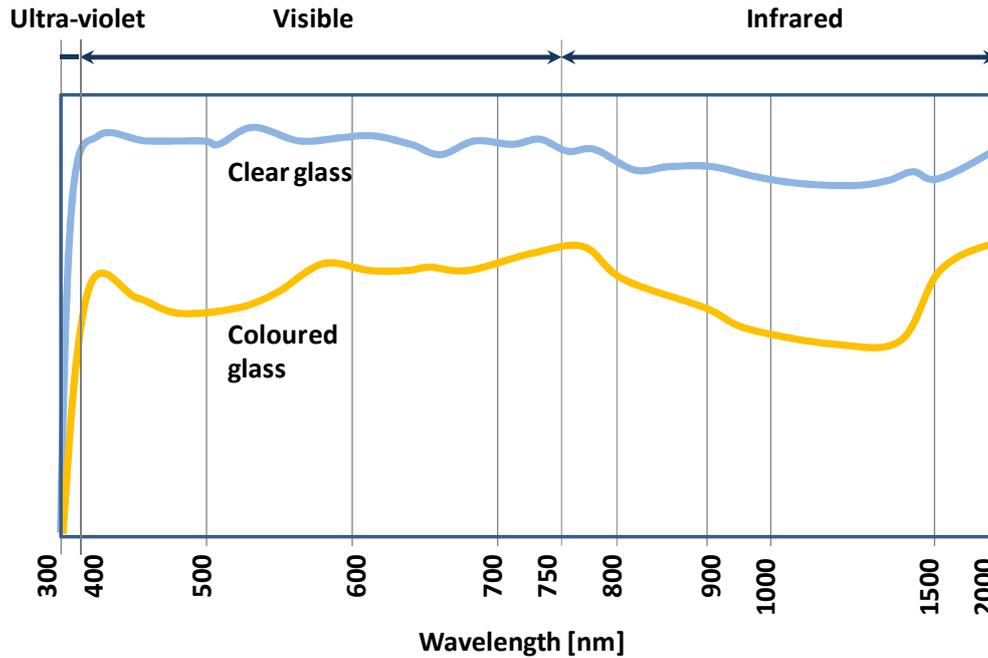
Figure 9: Transmittance characteristics of different glazing systems with respect to wavelength
