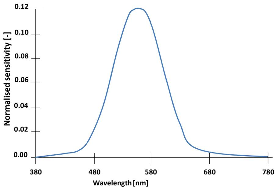
Figure 15: Response of human eye to the visible solar radiation spectrum
