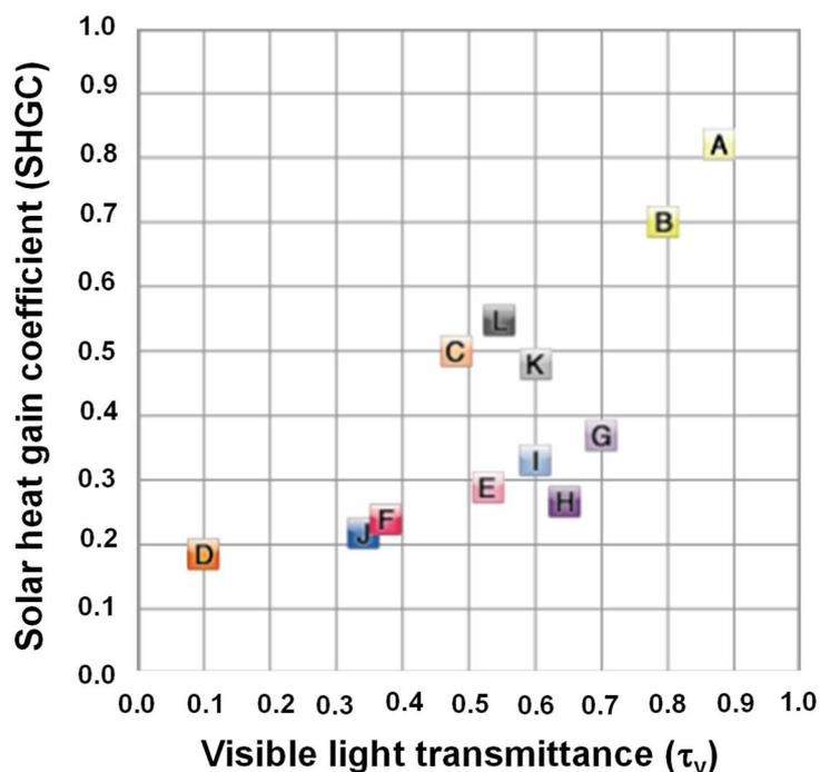
Figure 16: Visible light transmittance Vs. solar heat gain coefficient [25]
