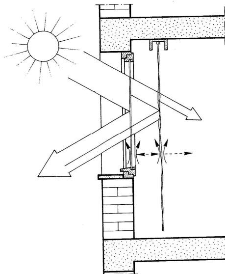
Figure 11: Thermal processes involved in the energy transmitted through a glazing surface [19]
