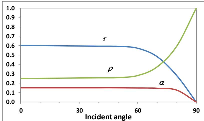
Figure 8: Transmission, sorption and reflection coefficients as a function of the incident angle
