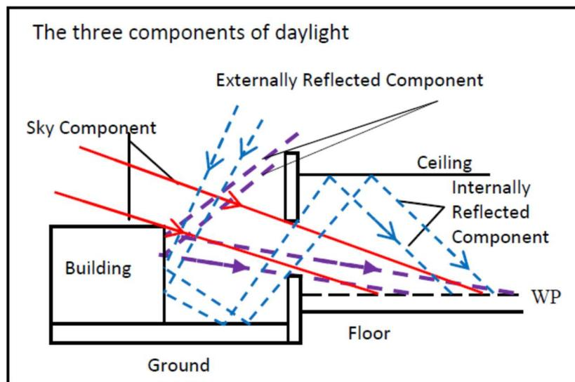
Figure 6. The three components of daylight: Sky Component (SC), Externally Reflected Component (ERC), Internally Reflected Component (IRC). [13]
