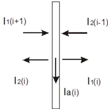
Figure 13: Radiation processes in a general  $i$ -th glazing element
