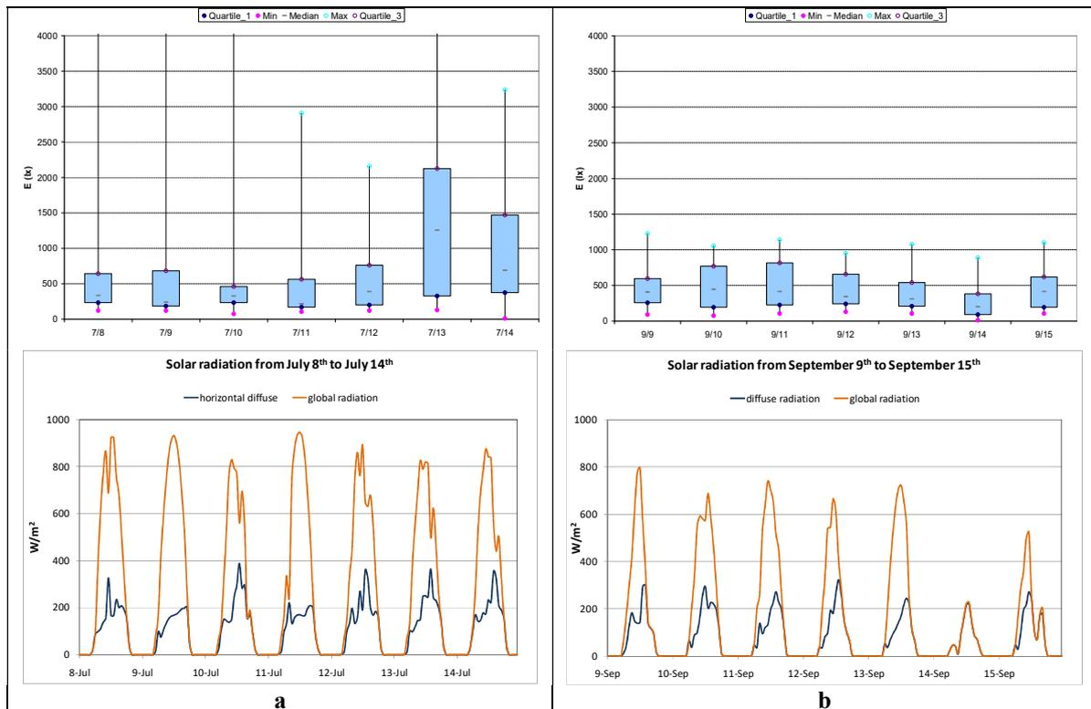
Figure 19: Comparison of illuminance values before (a) and after (b) film installation with the solar radiation for the considered periods
