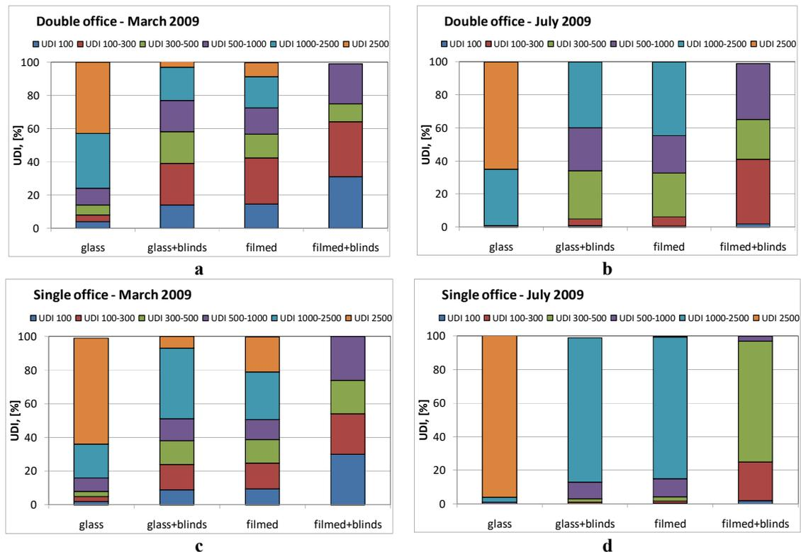
Figure 22 – UDI ranges, calculated for the year 2009, considering the situations for pre- and post-installation of the window film, for both roller blinds up and down conditions in a double office in March (a) and July (b) and in a single office in March (c) and July (d). Note that the orange colour indicates glare conditions
