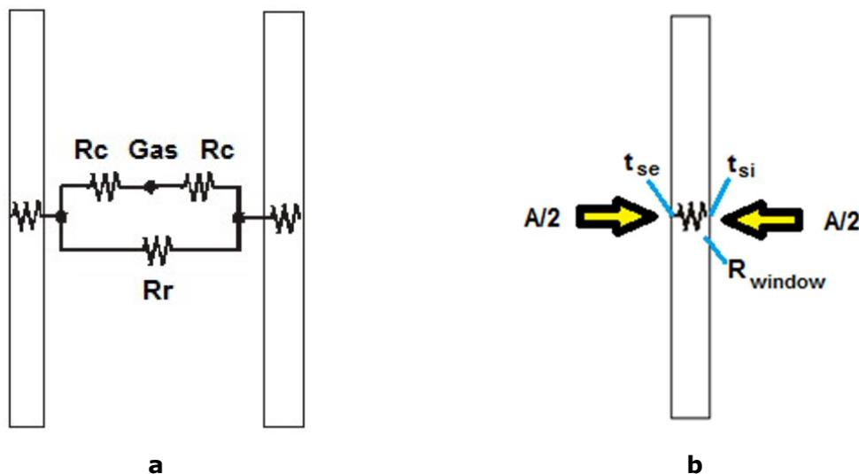
Figure 14: Possible schemes for determining window thermal balance
