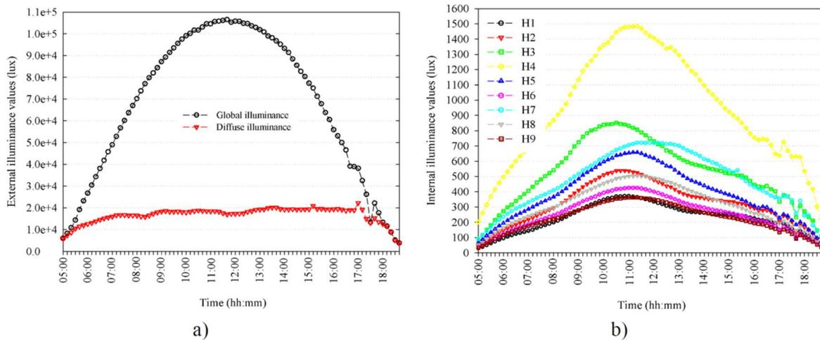
Figure 5. External diffuse and global horizontal illuminance values (a) and internal daylight illuminance values (b), both acquired on 18th June. [10]
