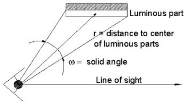
Figure 7. Explication of the parameters used for calculating the *UGR* [16]
