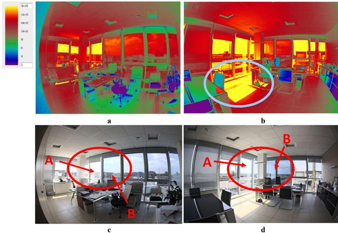
Figure 20: DR images of two offices taken during film application and false colour image which maps the luminance distribution within two rooms (a) and (b). Differences in the view to the outside resulting from film installation (c) and (d): "A" points existing glazing; "B" points filmed glazing
