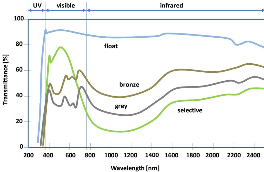
Figure 10: Transmittance characteristics of different glazing systems with respect to wavelength
