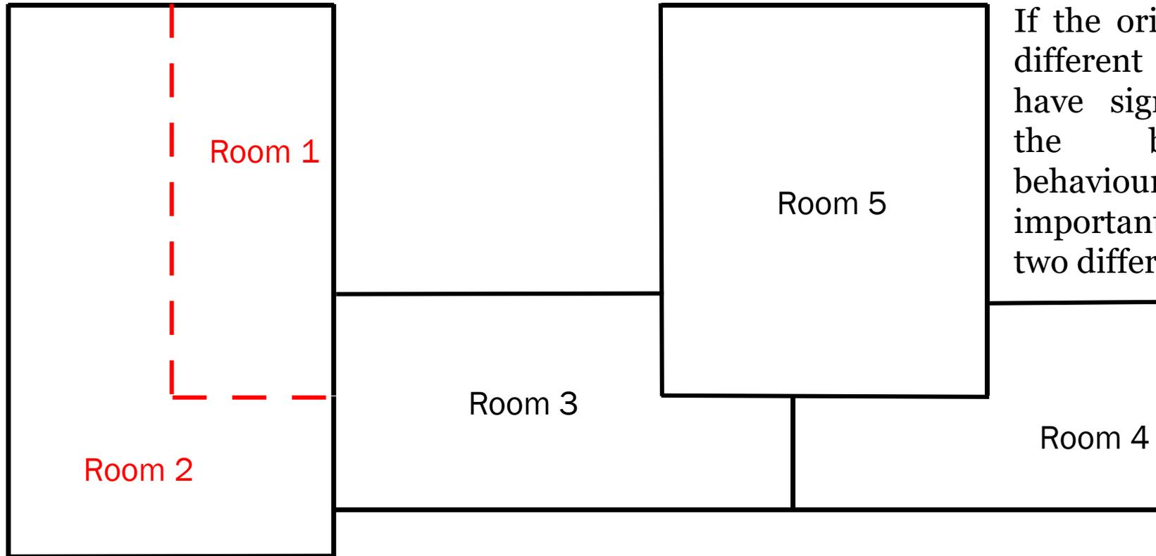
If the orientation is defined, different solar gains may have significant impact on the building energy behaviour, and it becomes important to split them in two different zones
