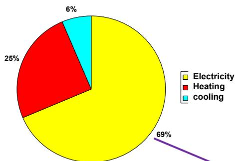
The diagram shows the average consumption (primary energy) of office buildings in the North of Italy. These values refer to the average office, i.e. with poor insulation.
