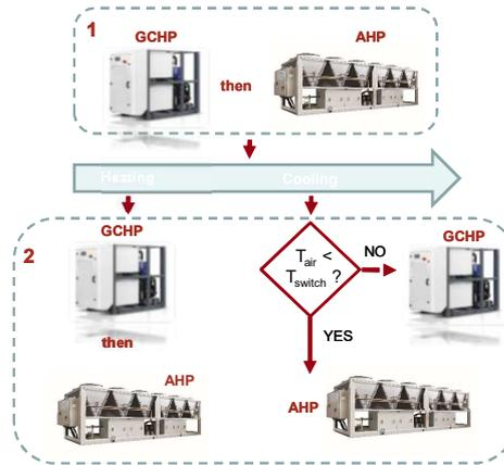
Using an **iterative procedure**, making use of computer simulations and the **load profile of this building**, the switch temperature resulted equal to **24°C**
