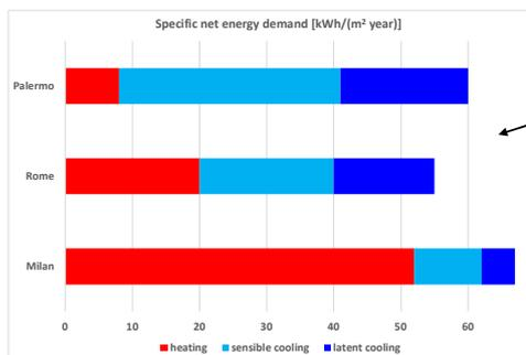
Example on the effect of the thermal inertia. The results show similar overall net energy demands in the 3 climates.
