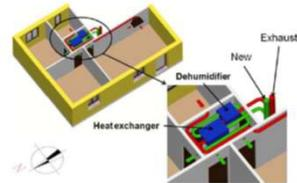
Case A: no dehumidification. Less energy need but no comfort in cooling season (dehumidification is needed in Italy)
