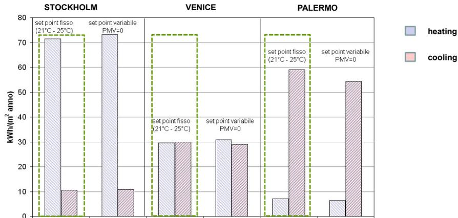
Building with glazed areas West and East oriented. Left bars are with fixed set-point. Right bars are with variable set-point as a function of comfort conditions.
