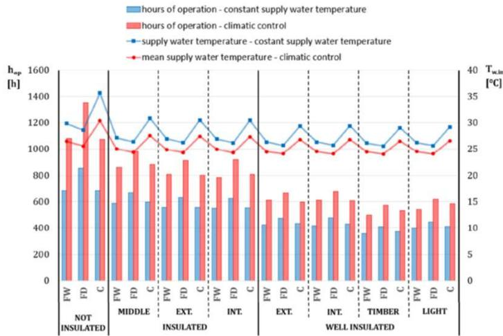
**Answer:** In new low energy/zero energy buildings you can choose any kind of radiant system. Running the system with a variable water temperature (supply temperature decrease when outside temperature increase) has a beneficial effect on the overall performance although the running hours (pumping energy costs) are higher
