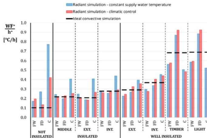
**Answer:** In new low energy/zero energy buildings it is not necessary to design and install low thermal inertia systems which may be more responsive. The overheating occurs because of the insulation of the building in any case (dot lines) even with an ideal convective system. The effect of a radiant system is negligible in the overheating, which is caused by good insulation and solar gains
