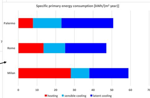
Example on the radiant ceiling coupled with dehumidified mechanical ventilation. The results show similar overall primary energy consumptions in the 3 climates.
