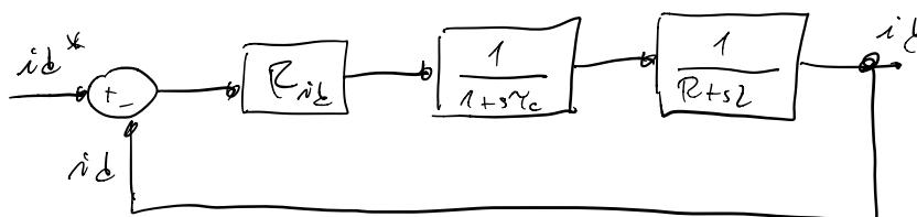
ESEMPIO : DIMENSIONARE ANOCCI DI CONTROLLO PER UN MOTORE SPM
