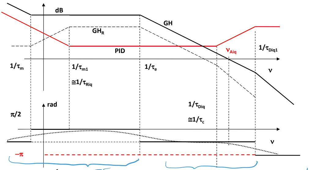
$$R_{Op} = k_i \frac{1+s\tau_{R,op}}{s} \underbrace{\frac{1+s\tau_{D,op}}{1+s\tau_{D,op1}}}_{PI} \quad D: Attenuazione banda passante$$
