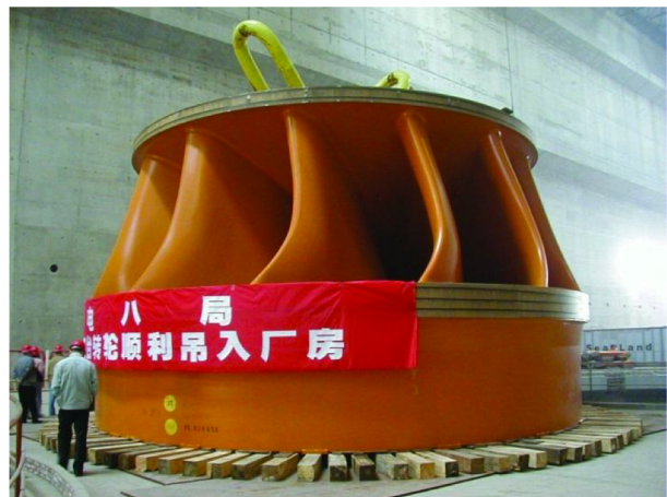
Three Gorges Dam, People's Republic of China Rated power output 700 MW per turbine Rated net head 80.6 m
