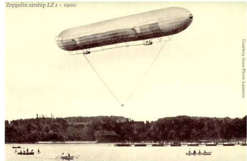
By sliding a weight suspended freely some 25 m below the LZ 1, the centre of gravity of the airship could be shifted. Thus elevation control was achieved.
