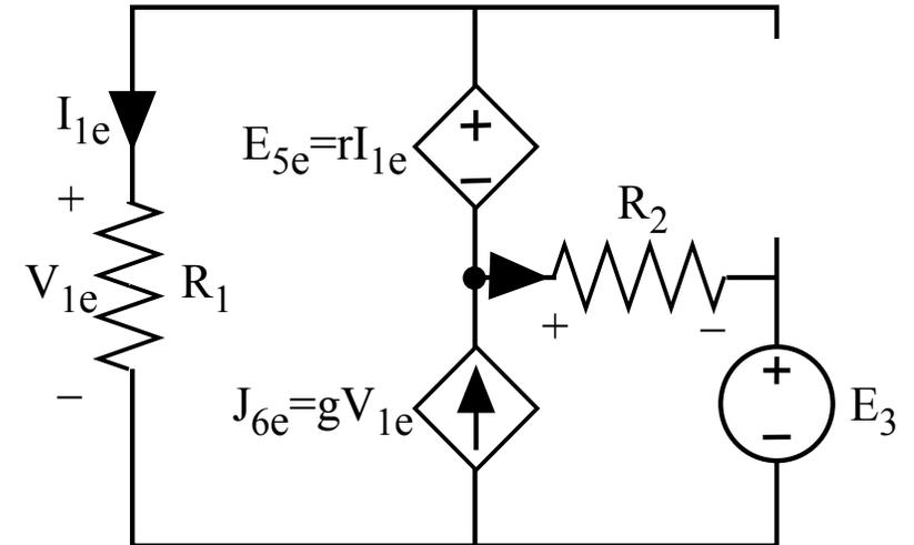
$$I_{1e} = \frac{1}{R_1 + R_2 - r - g R_1 R_2} E_3 = H_{G13} E_3 = 0,02 E_3$$
