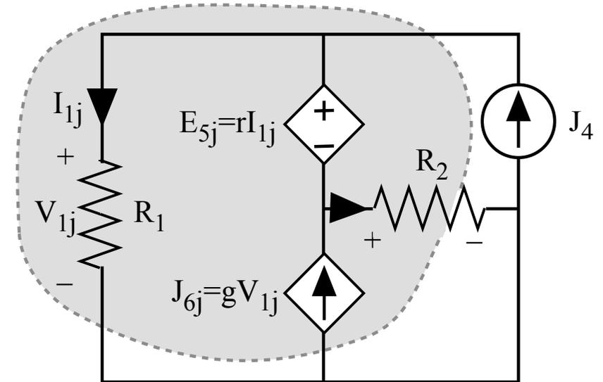
$$I_{1j} = \frac{R_2}{R_1 + R_2 - r - g R_1 R_2} J_4 = H_{I_{14}} J_4 = 0,1 J_4$$
