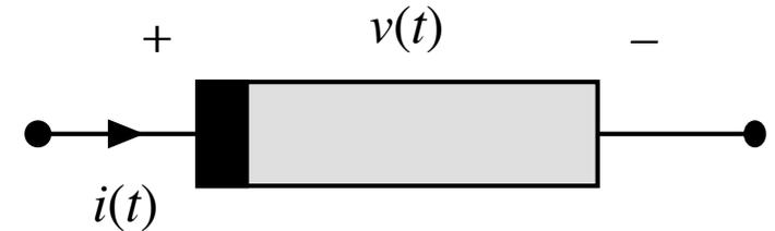
$$\begin{cases} v(t) = V_0 + \sum_{n=1}^{\infty} \sqrt{2} V_n \operatorname{sen}(n\omega t + \alpha_n) = V_0 + \sum_{n=1}^{\infty} v_n(t) \\ i(t) = I_0 + \sum_{n=1}^{\infty} \sqrt{2} I_n \operatorname{sen}(n\omega t + \beta_n) = I_0 + \sum_{n=1}^{\infty} i_n(t) \end{cases}$$
