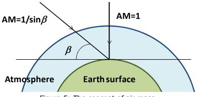
Figure 5: The concept of air mass.
