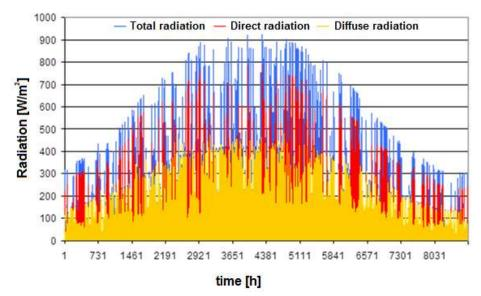
Figure 12: Example of solar radiation distribution over one year for the TRY of Venice
