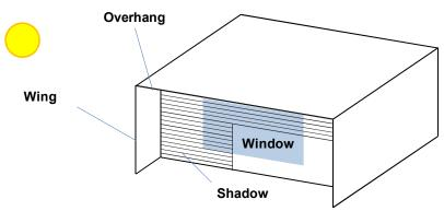
Figure 13: Example of architectural elements shading partially the building envelope
