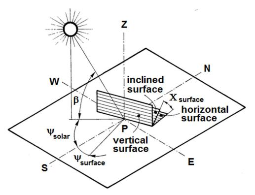
*Figure 8: Parameters defining the mutual position between the Sun and the generic surface of the building.*
