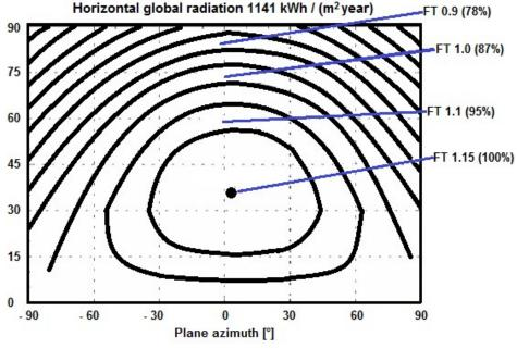
Figure 10: Example of Transposition Factor
