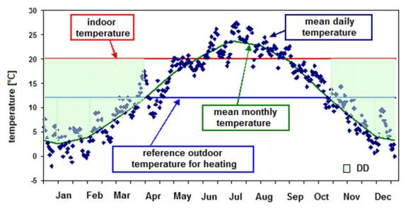
Figure 2: Graphical representation of the Heating Degree Days (HDD) of a typical year in Venice for an indoor temperature of 20°C and a threshold temperature for the outdoor air  $T_{threshold,heating} = 12°C$
