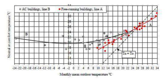
Figure 12: Finding s of Humphreys showing that in free-running buildings the expectations were different compared to air conditioned buildings in cooling [12].
