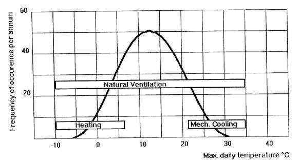
*Figure 19: Simplified explanation of the different approaches in cooling season to limit the indoor temperatures in a building. Source [14]*
