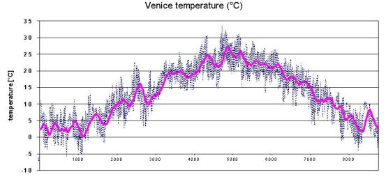
*Figure 17: Example of the weekly mean running temperature defined in EN 16798 considering the TRY of Venice*
