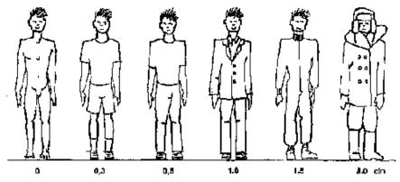
Figure 9: Insulation values of different kind of clothing (1 clo =  $0.155 \text{ m}^{2}K/W$ ). Source: [7]
