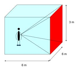
*Figure 4: Example of calculation of mean radiant temperature calculated in different locations in the room*
