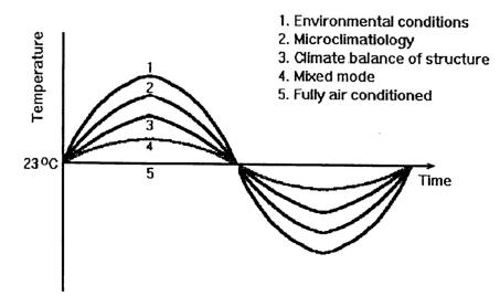
*Figure 18: Simplified explanation of the different approaches in cooling season to limit the indoor temperatures in a building. Source [14]*
