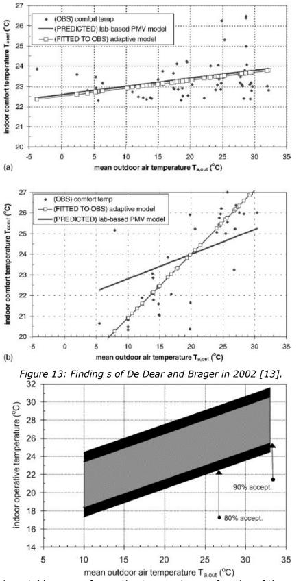
*Figure 14: Acceptable range of operative temperature as function of the mean monthly outdoor temperature. Source: [11]*
