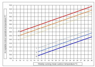
*Figure 15: Acceptable range of operative temperature as function of the weekly running mean outdoor temperature. Source: [9]*
