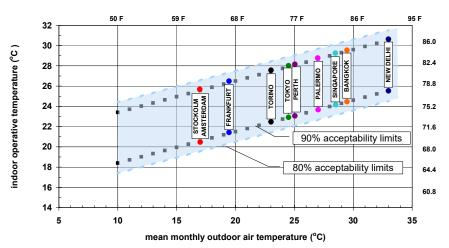
*Figure 16: Example of inner operative temperatures as a function of outdoor average temperature in the warmest month in different countries according to ASHRAE 55.*
