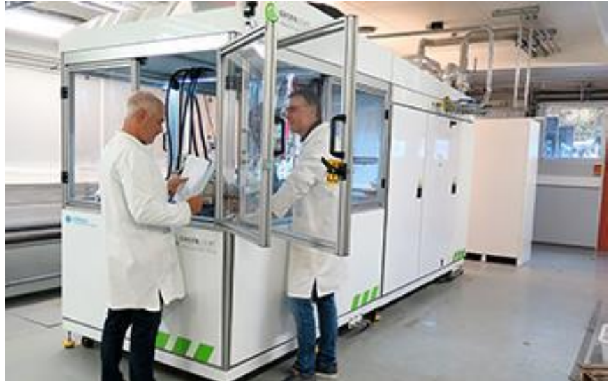
100 kW stack test bench
