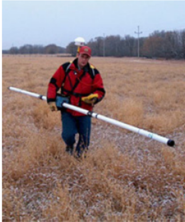
EM31 (Geonics), 9.8 kHz, s=3.66 m
