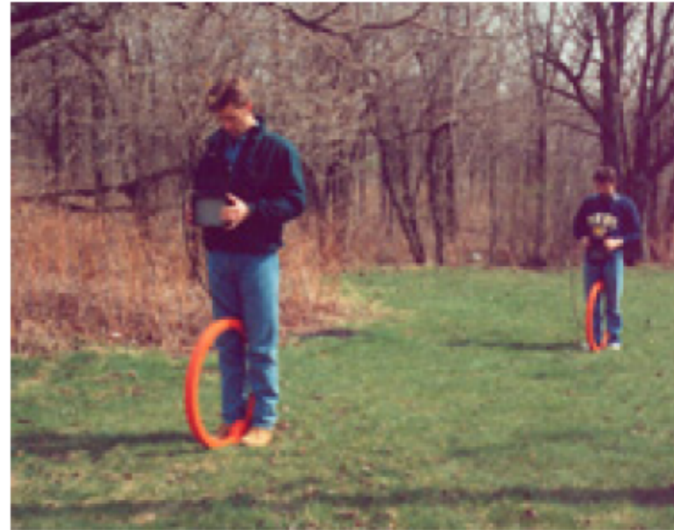
EM34 (Geonics), 6.4 kHz for s=10 m 1.6 kHz for s=20 m 0.4 kHz for s=40 m
