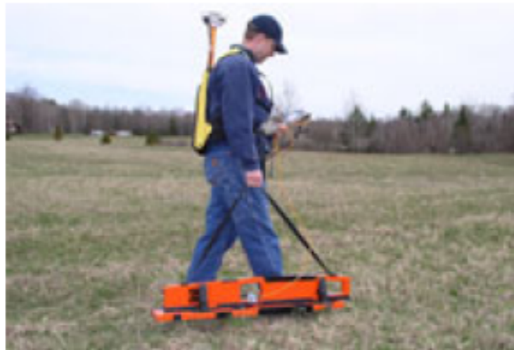
EM38 (Geonics), 14.6 kHz, s=1 m
