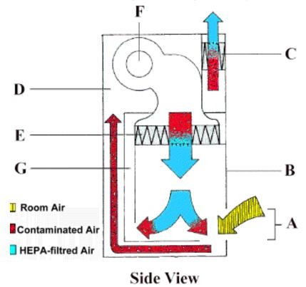
Class II, Type B2 (Connection to building exhaust system required.)
