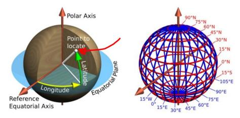
So the conventional reference frame has origin at the earth center, one axis is the rotational center, another axis passes. Greenwich coincident with the equator, and the other is consequently orthogonale (90°).
