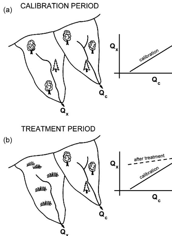
Fig. 1. Sketch of a paired-watershed experiment (from Hewlett, 1982).
