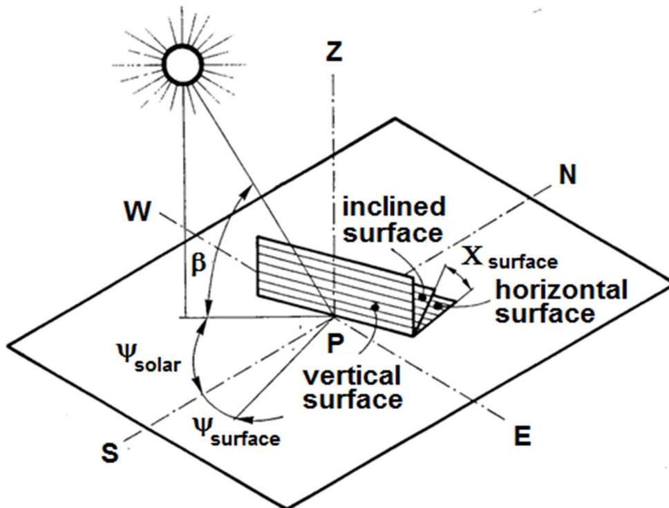
Figure 8: Parameters defining the mutual position between the Sun and the generic surface of the building.
