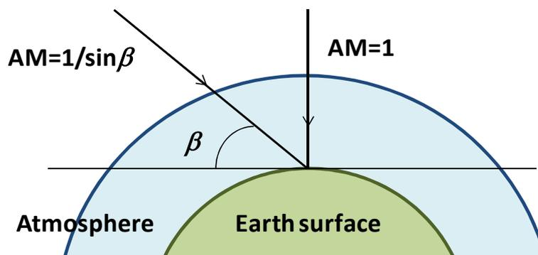
Figure 5: The concept of air mass.
