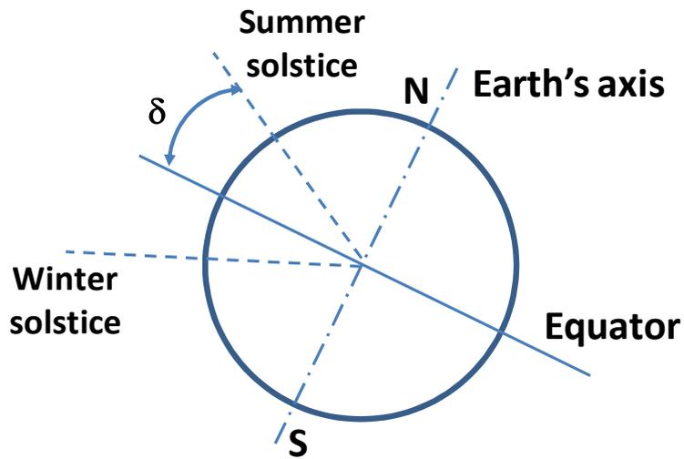
Figure 7: Parameters defining the mutual position between the Sun and the generic location on the Earth.
