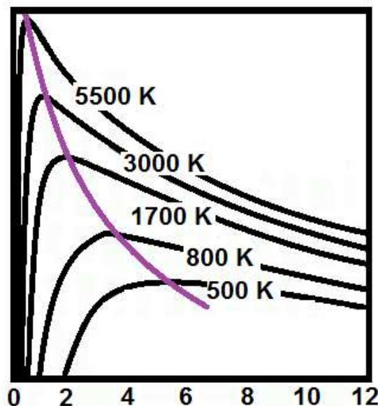
Figure 5: Radiation emission as a function of the wavelength [ $\mu\text{m}$ ] and absolute temperature of a black body
