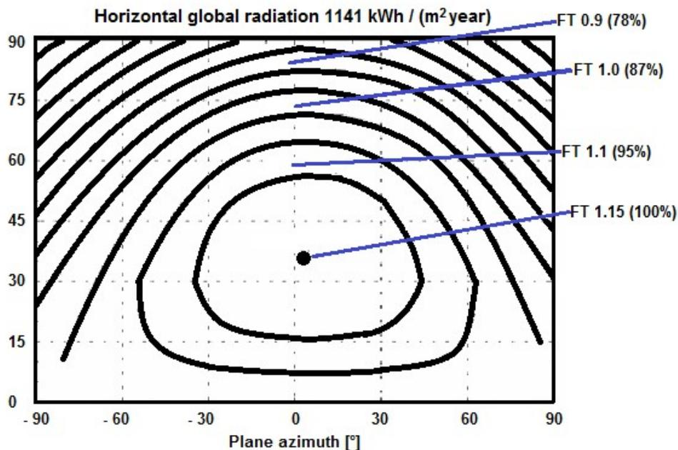
Figure 10: Example of Transposition Factor
