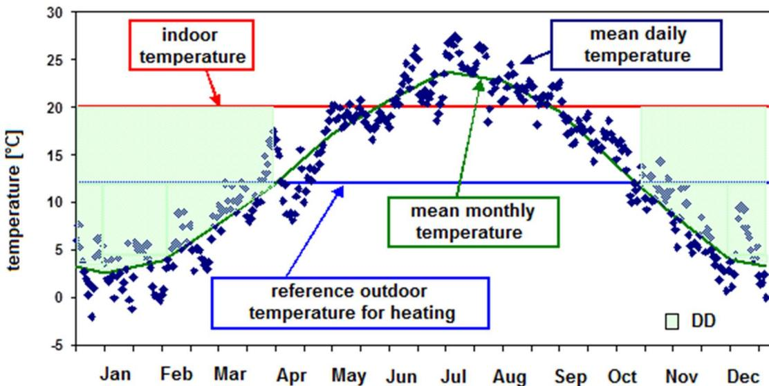
Figure 2: Graphical representation of the Heating Degree Days (HDD) of a typical year in Venice for an indoor temperature of 20°C and a threshold temperature for the outdoor air  $T_{threshold,heating} = 12^\circ\text{C}$
