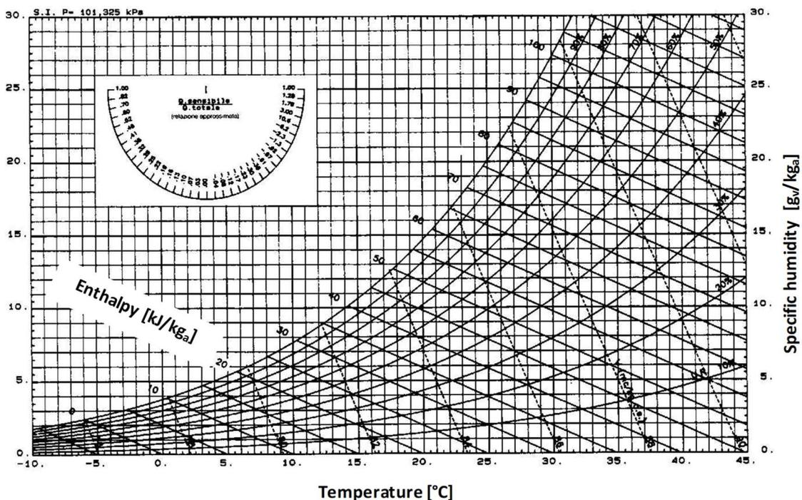
Figure 16: Diagram expressing relationship between air temperature and absolute humidity
