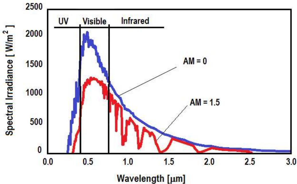
Figure 6: Spectral irradiance outside the atmosphere ( $AM=0$ ) and after a path with  $AM=1.5$  at sea level.
