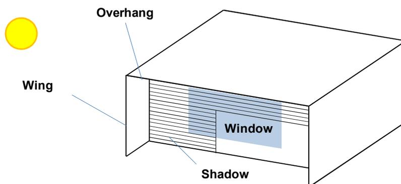
Figure 13: Example of architectural elements shading partially the building envelope
