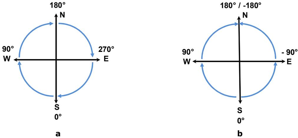
Figure 9: Usual definition of solar azimuth angle in a building simulation software.
