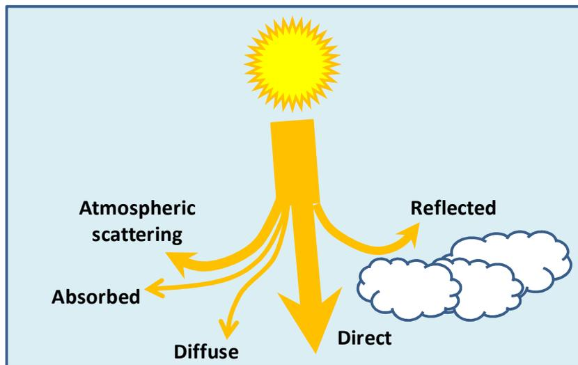
Figure 4: Phenomena involved in the solar radiation transmission through the atmosphere.
