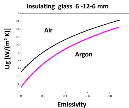
Thermal transmittance of double and triple glazing filled with different gases for vertical glazing
