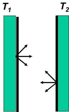
Plane, parallel, front facing surfaces at temperature, respectively,  $T_1$  and  $T_2$
